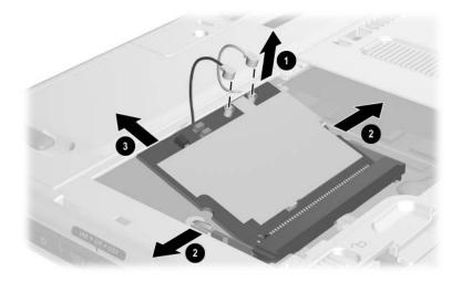
Removing the Mini PCI Communications Board
